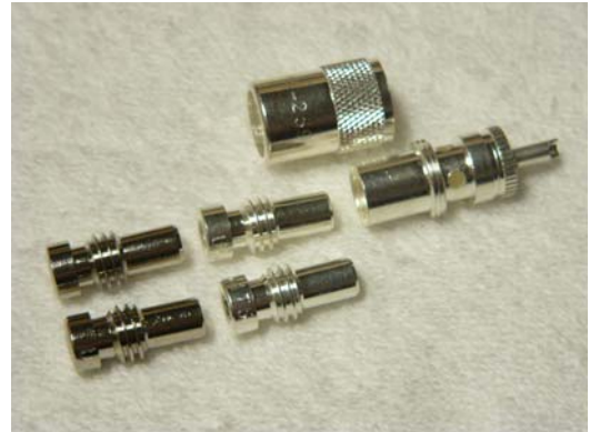
Soldering PL-259 connectors
